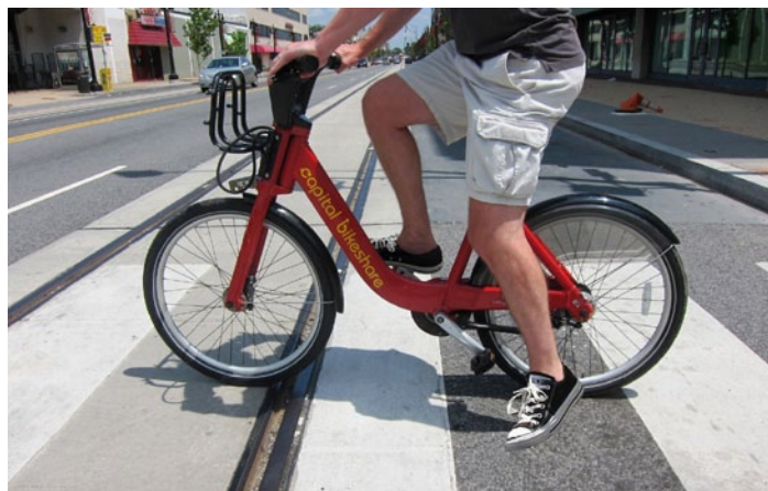
Below: A Capital Bikeshare user demonstrates safe right-angle crossing on streetcar tracks
